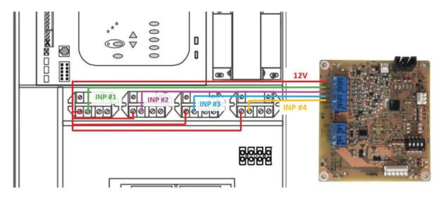
Typical example of wiring. Actual wiring may vary depending on controller manufacturer design and schematics. Installer must verify proper wiring with manufacturer of system controller. Waterway does not assume responsibility for any miswiring.
