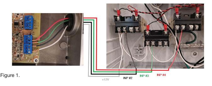
Typical Connection using 3 relays to control INP #2, INP #3, and INP #4
