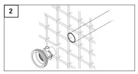
2. Estimate needed length of 2" PVC pipe by thickness of wall and length of jet body (5.87").
