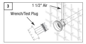
3. Glue the jet body onto the end of the pipe and ½" PVC for air line (3 ¾" behind face) for pressure test before guniting. Use Wrench to plug the body for pressure test.
