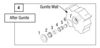
4. After guniting, install the internal components of the jet. Improper re-assembly will inhibit function of the jet.
