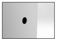
1. Locate a flat surface on the spa wall to install the Micro Component. Drill a 43/64" hole through the spa wall. Clean debris around the hole on the front and back.
