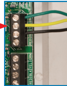
Figure 12. Jandy Pro Series VSP Connection to Pump
