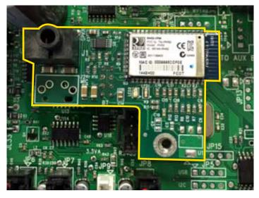
4. Secure the Bluetooth circuit board with a #6-32 screw.
