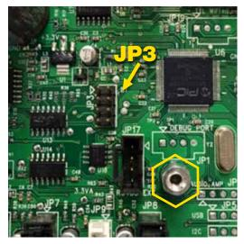
**3.** Install Bluetooth circuit board. Connector JP3 should mate with the Bluetooth circuit board.
