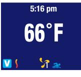
Press the SWIM button to turn the pump ON – the blue SWIM icon on the LCD screen turns ON.
