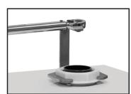
4. Apply the nut and hand tighten, then torque the nut to specifiction.
