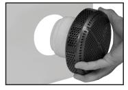
2. Insert the suction wall fitting with gasket through the hole of the spa. No spot facing or silicone is necessary.
