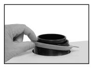
3. Ensuring the fitting with gasket are flat against the spa wall and centered within the hole, add the Load Washer ring to the back so the cone locates into the hole.
