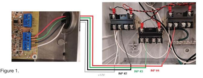
Typical Connection using 3 relays to control INP #2, INP #3, and INP #4 **NOTE:** +12v is jumped to each relay
