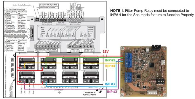
Typical example of wiring. Actual wiring may vary depending on controller manufacturer design and schematics. Installer must verify proper wiring with manufacturer of system controller. Waterway does not assume responsibility for any miswiring.
