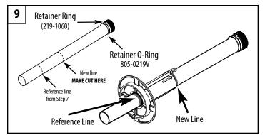
9. Remove the 1" pipe assembly from the jet body assembly and realign the measuring tool with the reference line. Make a new line at the Poly Storm Gunite Jet setback on the measuring tool.
