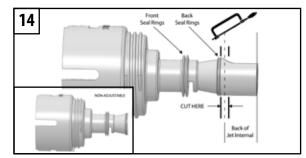
14. To make a non-adjustable jet internal, cut off the back of the jet internal after the back seal rings.
