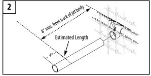
2. Estimate needed length of 2  $\frac{1}{2}$ " PVC pipe by thickness of wall. Cut 2  $\frac{1}{2}$ " PVC pipe at least 4" longer than estimated finish length. Then glue 2  $\frac{1}{2}$ " PVC pipe to body.
