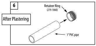
6. Cut a piece of 1" PVC pipe few inches longer than the 2  $\frac{1}{2}$ " pipe and glue the threaded retainer ring to one end.
