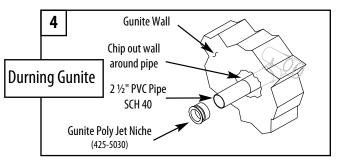
4. While guniting, scoop out gunite around the 2  $\frac{1}{2}$ " PVC pipe, allowing room for the plaster niche (425-5030).
