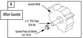
5. Before plastering, cut the  $2 \frac{1}{2}$ " pipe so that the plastic niche will fit flush with the finished wall. Glue the plaster niche onto the pipe, then cover the niche with tape for plastering.
