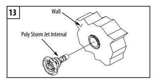
13. Insert Poly Storm Internal into the wall fitting and thread in passed first stop. Do not force. To reduce water flow, turn clockwise. To increase water flow, turn counter-clockwise until it stops turning. To remove, continue turning counter-clockwise past the stopping point. You will hear a snap to confirm release of Poly Storm internal.
