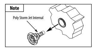
Note: To winterize the jet system, remove the jet internal from the wall fitting ONLY. Install a #10 rubber expansion plug inside of the fitting opening.
