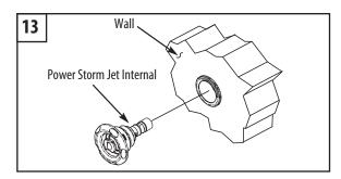
14. Insert Power Storm Internal into the wall fitting and thread in passed first stop. Do not force. To reduce water flow, turn clockwise. To increase water flow, turn counter-clockwise until it stops turning. To remove, continue turning counter-clockwise past the stopping point. You will hear a snap to confirm release of Power Storm internal.
