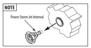
Note: To winterize the jet system, unthread the jet internal from the wall fitting ONLY. Install a #10 rubber expansion plug inside of the fitting opening.
