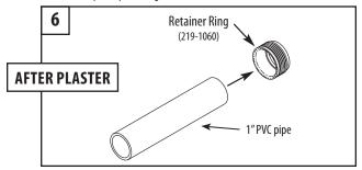
6. Cut a piece of 1" PVC pipe a couple of inches longer than the 2  $\frac{1}{2}$ " pipe and glue the threaded retainer ring to it.
