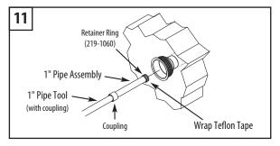
11. Install 4-6 wraps of Teflon tape around the threaded Retainer Ring, including 1 wrap over the 0-Ring. Dry fit the pipe tool with coupling on the end of the 1" pipe assembly. Thread the assembly into the body assembly until it is snug and the pipe tool with coupling spins freely. Remove the pipe tool from the end of the pipe assembly.
