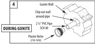
4. While guniting, scoop out gunite around the 2  $\frac{1}{2}$ " PVC pipe, allowing for the plaster niche (218-7650).
