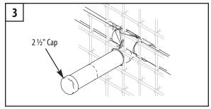
3. Glue 2 ½" cap onto end of pipe for pressure test, before guniting.
