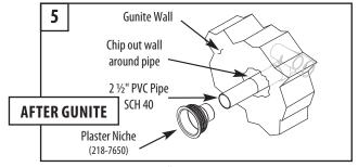
5. Before plastering, cut the 2 ½" pipe so that theplastic niche will fit flush with the finished wall. Glue the plaster niche onto the pipe, then cover the niche with tape for plastering.
