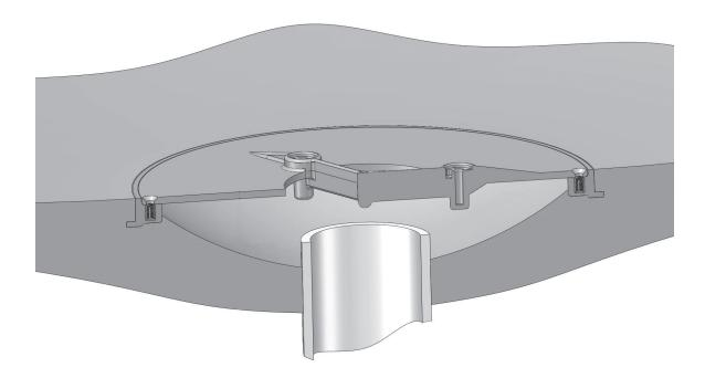
**NOTE:** For fastener repair, evaluation and replacement - if any of the listed fastener or fastener receptacles in these instructions are damaged in any manner such that that the required torque specification cannot be achieved, both the fastener and receptacle parts must be replaced
