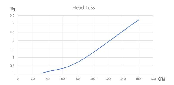
2" Connection: measured 15" downstream of the 90°elbow that was directly attached to the 'sump' (in this case, the fittings used to create an open pipe placed 1" below the bottom of the adapter plate); 2" sch 40 PVC
