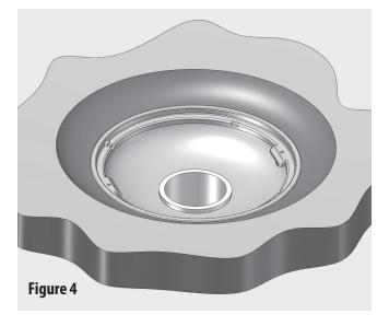
4. Align the drain cover support plate (#8) over the ring or sump (Figure 5). The top of the outlet pipe should be recessed a minimum of 1 inch from the back of the plate (Figure 6).
