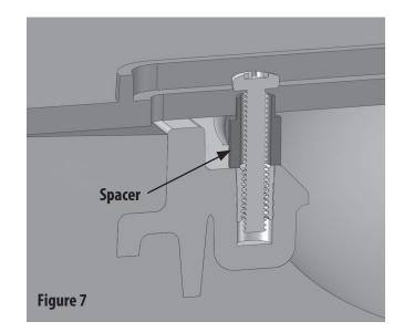
**NOTE:** For fastener repair, evaluation and replacement - if any of the listed fastener or fastener receptacles in these instructions are damaged in any manner such that the required torque specification cannot be achieved, both the fastener and receptacle parts must be replaced
