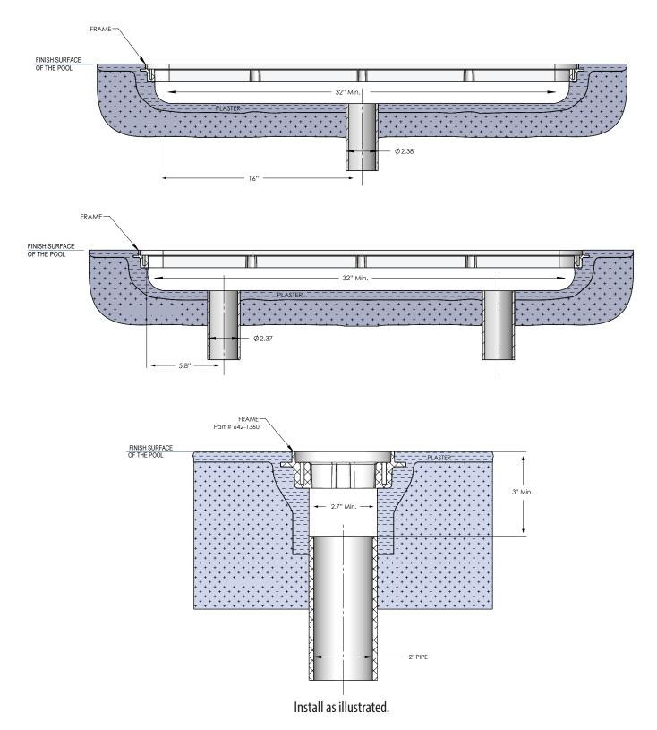
NOTE: No reductions in plumbing size are permitted within 16" from the point of connection to the sump.
