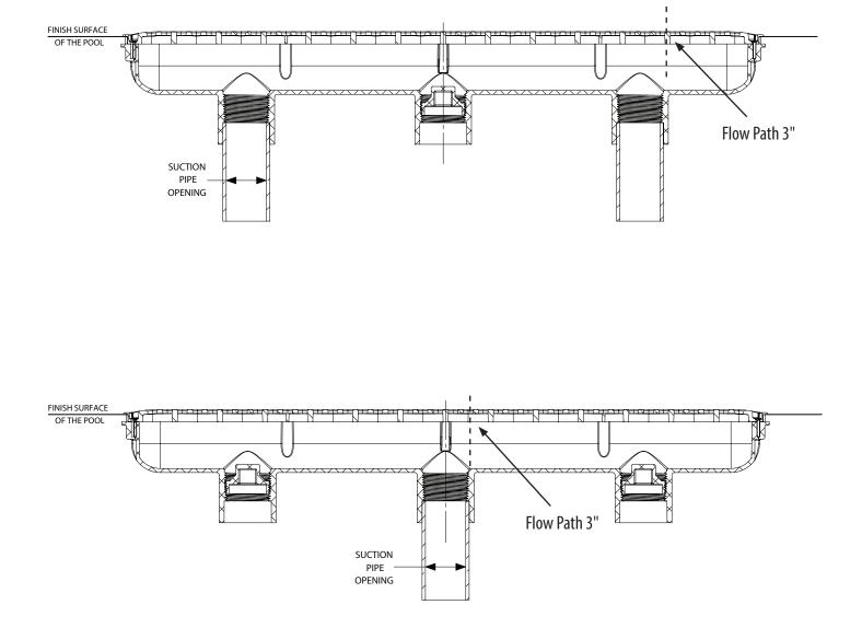
NOTE: No reductions in plumbing size are permitted within 16" from the point of connection to the sump.
