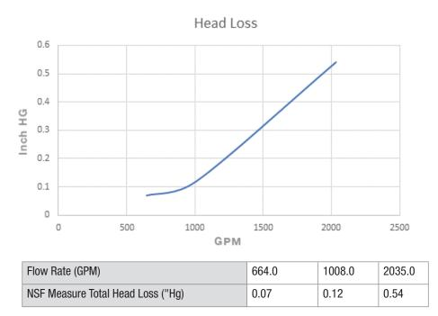
Pressure Tap located downstream of 2 schedule 40 10" elbows and an 8.25" length of straight 10" pipe.
