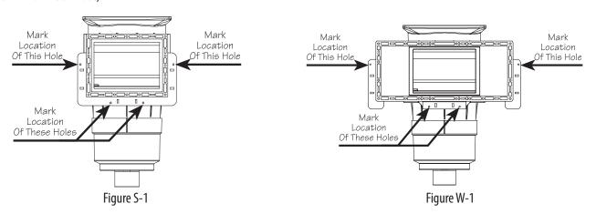
4. Remove the skimmer and drill 7/32" diameter holes in the locations you marked in step #3.
