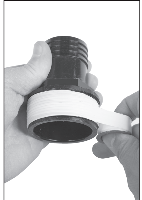
3. Wrap 4 turns of Teflon tape on 417-6161 hose adaptor.
