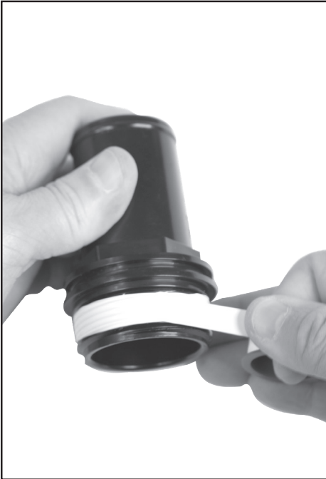
1. Wrap 4 turns of Teflon tape on 417-6141 hose adaptor.
