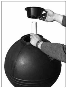
2. Place sand filter guide in filter over stand pipe. Add approximately 3 inches of water before adding sand. Add required #20 grade silica sand (see sand chart on back page). Remove sand filter guide and save.
