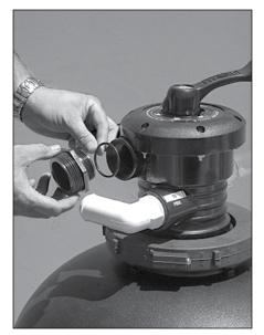
Take O-ring and put over small side threads on 1 ½" buttress x MPT fitting. Thread onto pump outlet on multi-port valve (top port).
