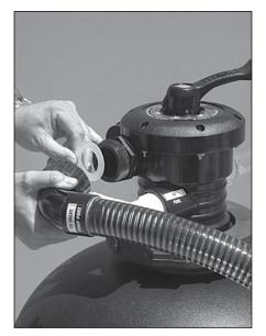
10. Install other end of pump hose labeled "TO VALVE PUMP PORT" by putting 1 ½" gasket into nut (smaller end) and threading onto buttress x MPT fitting. DO NOT OVER TIGHTEN.
