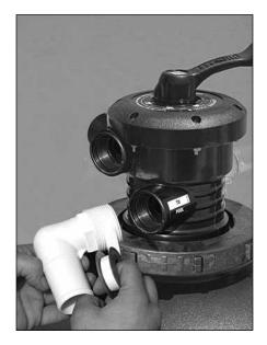
6. Apply Teflon tape to 90° smooth hose adapter threads (4 wraps) and and thread into the bottom of the multi-port (to pool).
