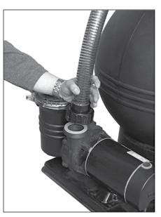
Put 2" gasket into nut (larger end) on hose labeled "TO VALVE PUMP PORT." DO NOT OVER TIGHTEN.
