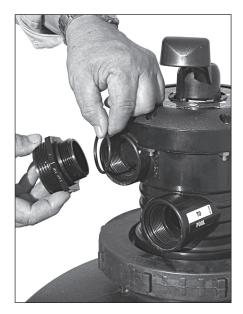
8. Take O-ring and put over small side threads on 1 1/2" buttress x MPT fitting. Thread into pool outlet on valve. Repeat for pump outlet on valve.
