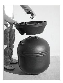
Attach filter base to filter body by turning body upside down. Align drain on filter with clearance slot on base. Slip washer over bolt and thread bolt into filter body. DO NOT OVER TIGHTEN.
