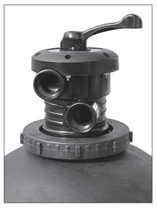
Split-nut is fully installed when threads on body are not exposed. Retighten bolt on split-nut.
