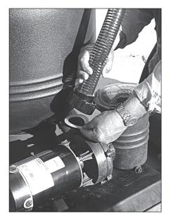
11. Put 2" gasket into nut on hose labeled "TO VALVE PUMP PORT." DO NOT OVER TIGHTEN.
