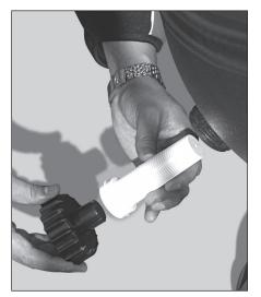
16. To remove drain screen, remove drain screen cap/wrench and insert the wrench end into drain screen opening and unscrew. When reinserting drain screen DO NOT OVER TIGHTEN (be sure 0-ring is inside of drain cap). Screw on drain screen cap/wrench. DO NOT OVER TIGHTEN.
