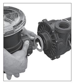
Install trap base to pump by removing gasket from inside trap. Remove clear trap lid, and place gasket in trap nut. Thread onto pump. DO NOT OVER TIGHTEN. Place pump with trap onto pump base. Remember to replace trap lid.
