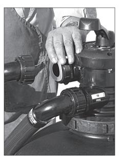
**10.** Take pump to filter hose assembly and put 1 ½" gasket into nut on smaller end with sweep 90°. Thread onto pump outlet port. **DO NOT OVER TIGHTEN**.
