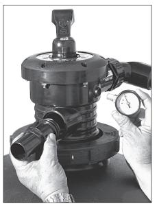
**13**. Apply Teflon tape to pressure gauge threads (4 wraps is ideal) and thread into valve. Install waste adapter by pushing O-ring over threads of adapter and threading into waste port.
