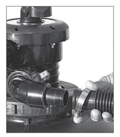
Install hose onto smooth hose adapter in valve by loosening hose clamp and sliding over adapter end. Install other end onto return fitting of pool and tighten clamps.
