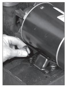
7. Install anchors into slots of pump, and then into the holes in the pump base. Push pins into anchors to secure.
