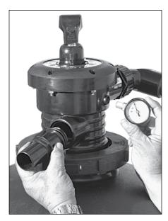
13. Apply Teflon tape to pressure gauge threads (4 wraps is ideal) and thread into valve. Install waste adapter by pushing 0-ring over threads of adapter and threading into waste port.
