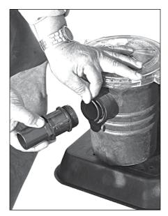
**12.** Put O-ring over threads on 1 ½" smooth straight hose adapter and thread into front of pump basket.
