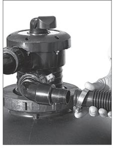
**14.** Install hose onto smooth hose adapter in valve by loosening hose clamp and sliding over adapter end. Install other end onto return fitting of pool and tighten clamps.
