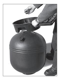
Attach filter base to filter body by turning body upside down. Align drain on filter with clearance slot on base. Slip washer over bolt and thread bolt into filter body.
