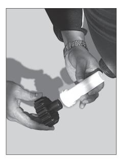
To remove drain screen, remove drain screen cap/wrench and insert the wrench end into drain screen opening and unscrew. When reinserting drain screen DO NOT OVER TIGHTEN (be sure 0-ring is inside of drain cap). Screw on drain screen cap/wrench. DO NOT OVER TIGHTEN.
