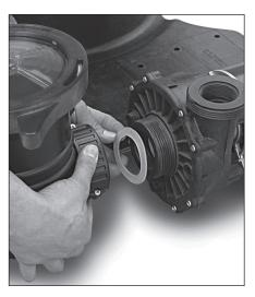
Install trap base to pump by removing gasket from inside trap. Remove clear trap lid, and place gasket in trap nut. Thread onto pump.
