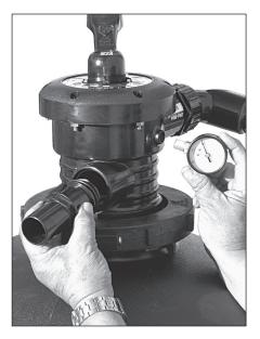
Apply Teflon tape to pressure gauge threads (4 wraps is ideal) and thread into valve. Install waste adapter by pushing O-ring over threads of adapter and threading into waste port.
