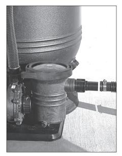
Install 6 ft. corrugated hoses by loosening hose clamps and sliding over hose ends. Install hose onto pump basket hose fitting by pushing on and tightening clamp. Install other end of hose onto skimmer and tighten clamp.
