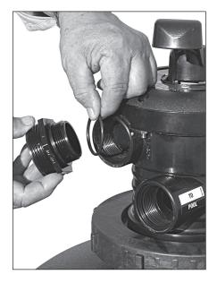
Take O-ring and put over small side threads on 1 <sup>1</sup>/<sub>2</sub>" buttress x MPT fitting. Thread into pool outlet on valve. Repeat for pump outlet on valve.
