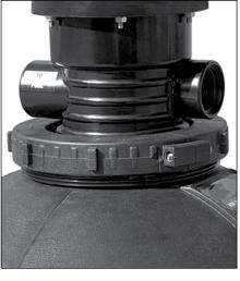
Place valve over threads on sand filter. Make sure dual outlets face pool and that top of filter is clear of any debris.
