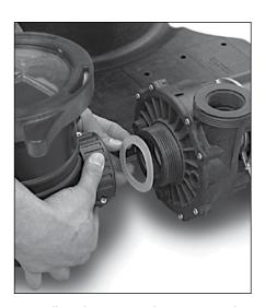
6. Install trap base to pump by removing gasket from inside trap. Remove clear trap lid, and place gasket in trap nut. Thread onto pump. DO NOT OVER TIGHTEN. Remember to replace trap lid.
