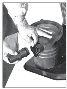
**11**. Put 0-ring over threads on 1 ½" smooth straight hose adapter and thread into front of pump basket.
