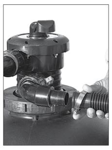
14. Install hose onto smooth hose adapter in valve by loosening hose clamp and sliding over adapter end. Install other end onto return fitting of pool and tighten clamps.
