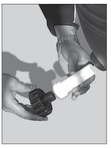
15. To remove drain screen, remove drain screen cap/wrench and insert the wrench end into drain screen opening and unscrew. When reinserting drain screen DO NOT OVER TIGHTEN (be sure 0-ring is inside of drain cap). Screw on drain screen cap/wrench. DO NOT OVER TIGHTEN.
