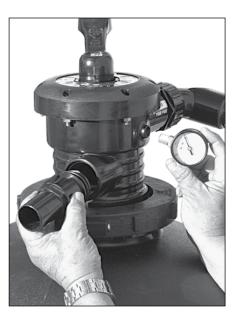
12. Apply Teflon tape to pressure gauge threads (4 wraps is ideal) and thread into valve. Install waste adapter by pushing O-ring over threads of adapter and threading into waste port.
