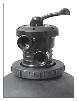
**5**. Split-nut is fully installed when threads on body are not exposed. Retighten bolt on split-nut after installation to ensure valve is not loose.
