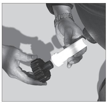
6. To remove drain screen, remove drain screen cap/wrench and using the wrench end, insert into drain screen opening and unscrew. When reinserting drain screen DO NOT OVER TIGHTEN (be sure 0-ring is inside of drain cap). Screw on drain screen cap/wrench. DO NOT OVER TIGHTEN.
