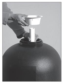
2. Turn filter over. Place next to pool between skimmer and return opening on pool. Place sand filter guide in filter over stand pipe. Fill tank approximately ¾ full of water before adding sand. Add required #20 grade silica sand (see sand chart on back page). Remove sand fill guide and save.
