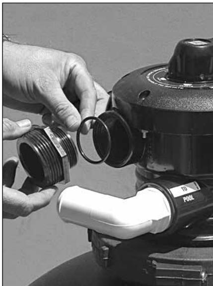
7. Take O-ring and put over small side threads on 1 ½" buttress x MPT fitting. Thread onto pump outlet on multi-port valve (top port).
