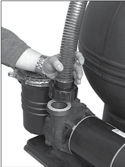
9. Put 2" gasket into nut (larger end) on hose labeled "TO VALVE PUMP PORT". **DO NOT OVER TIGHTEN.**
