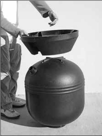
1. Attach filter base to filter body by turning body upside down. Align drain on filter with clearance slot on base. Slip washer over bolt and thread bolt into filter body. **DO NOT OVER TIGHTEN.**
