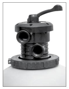
Split-nut is fully installed when threads on body are not exposed. Retighten bolt on split-nut after installation to ensure valve is not loose.
