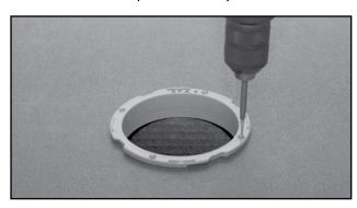
4. Screw the wall fitting to the spa wall using the four #6 x 1" oval Phillips-head screws.
