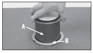
5. Aligning the groove in the speaker body (A) with the tab (B) inside the wall fitting, slide the speaker body through the wall fitting until it lies flush on the flange hole.
