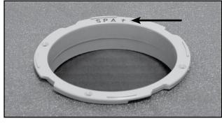
2. Place the wall fitting in the 47/8" hole and position the "SPA"/arrow in toward the inside of the spa as indicated by arrow.
