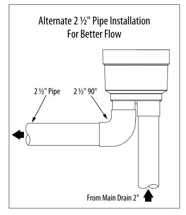
For 1  $\frac{1}{2}$ " or FPT Skimmer (2" Spigot) beat results are 1  $\frac{1}{2}$ " pipe to drain and 2" 90° for pump.
