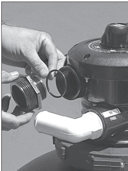
7. Take O-ring and put over small side threads on 1 1/2" buttress x MPT fitting. Thread onto pump outlet on multi-port valve (top port).
