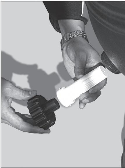
5. To remove drain screen, remove drain screen cap/wrench and insert the wrench end into the drain screen opening and unscrew. When reinserting drain screen **DO NOT OVER TIGHTEN** (be sure O-ring is inside of drain cap). Screw on drain screen cap/wrench. **DO NOT OVER TIGHTEN.**
