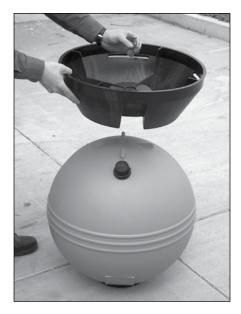
Attach filter body onto filter base by turning body upside down. Align drain on filter with clearance slot on base. Slip washer over bolt and thread bolt into filter body. DO NOT OVER TIGHTEN.
