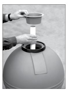
2. Turn filter over and place sand fill guide in filter over stand pipe. Fill with water before adding sand. Add required #20 grade silica sand (see sand chart). Remove sand fill guide and save.
